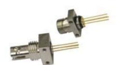
The MLD2315-4x5 uses a high-performance laser diode designed to meet performance requirements for 500Mbps data communication over multimode optical fiber. Applications include Ethernet, Fiber Channel and ATM protocols. The optical assembly is designed to interface either 50um or 62.5um multimode fiber
